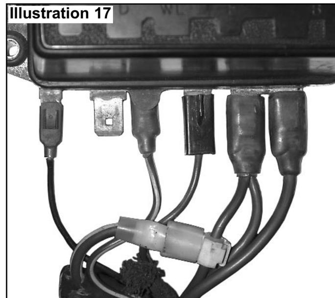
Remove the Brown/Green wire from the "F" terminal and cut off the spade connector with a set of wire cutters. Strip the wire so that about 1/4" of insulation is removed. (Illustration 18)
