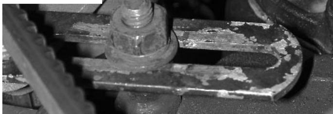
2. Remove the pivot bolts from the water pump ear and the rear mounting bracket using a 1/2" wrench and 1/2" socket.
