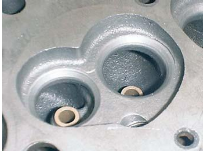
The deep, closed style combustion chambers characteristic of all the earlier heads as seen in this photo.
