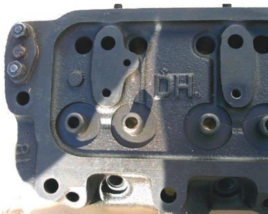
The casting number is located further forward on the cylinder head than in previous models as seen here.
