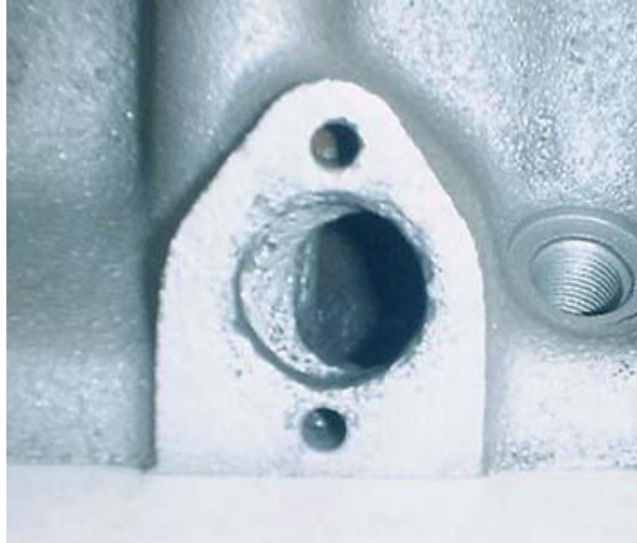
With heads 2923 and on, the hole for the heater port was enlarged. Our assumption is this hole was made bigger to help facilitate the removal of casting sand. The hole in the heater valve is smaller than either of these, so it shouldn't have anything to do with coolant flow.
