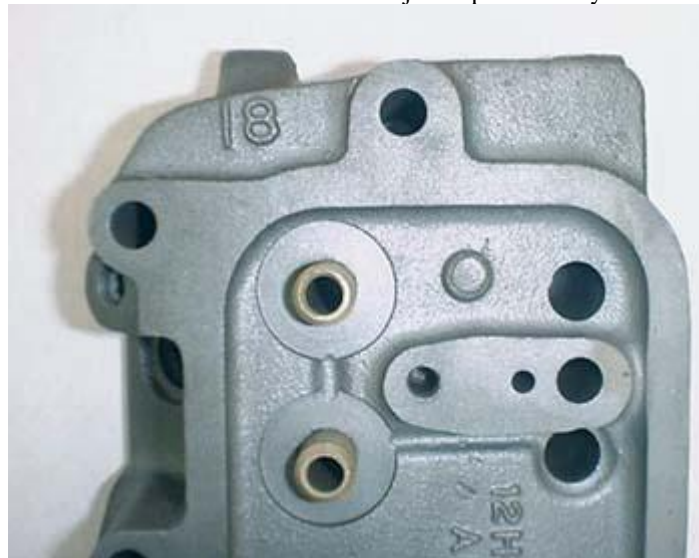
2389's also have 18 cast in rear to denote 1800cc engine size, again the air injector hole is obvious at upper left.
