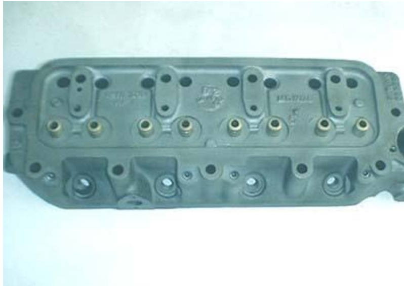
2389 heads were the first to come with the air injector ports clearly visible in this photo.
