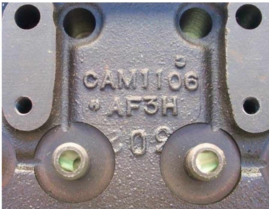
The casting number is located further forward on the cylinder head than in previous models as seen here.
