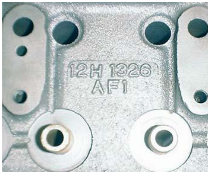
The casting number is seen in the above photo along with the in-line oil feed hole for the rocker shaft.
