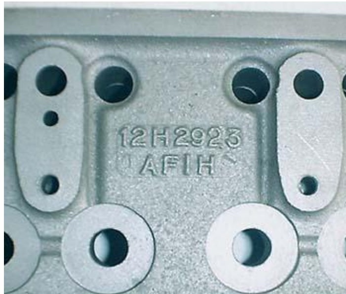
The casting number is seen in the above photo along with the in-line oil feed hole for the rocker shaft.
